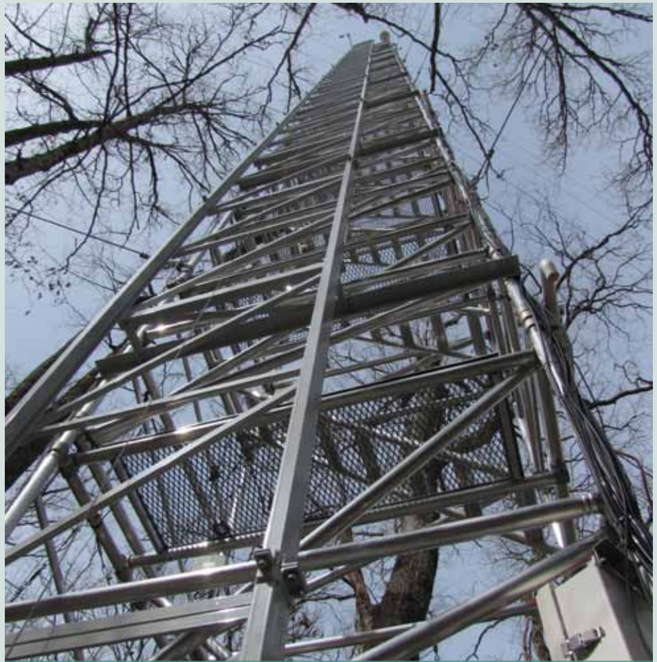
Eddy covariance tower installed last year at Coweeta to measure the flow of carbon dioxide and other gases above the forest canopy. The observations made with this system, which is separate from the RAFES system, are critical for detecting variations in carbon and nutrient gases in relation to climate change. (photo by Zoë Hoyle, USDA Forest Service)
