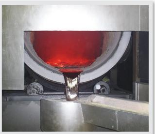
Scrap aluminum is melted to remove impurities.
