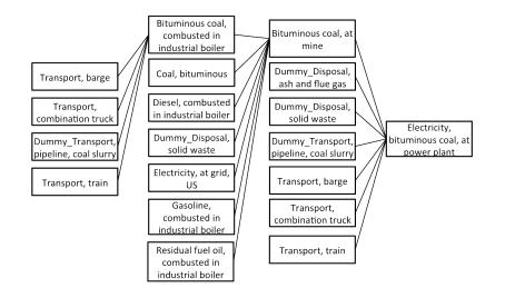
Figure 3: Partial map of unit processes associated with "Electricity, bituminous coal at power plant"
