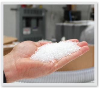
Small polypropylene pellets are packaged and shipped to manufacturing facilities that create plastic products.
